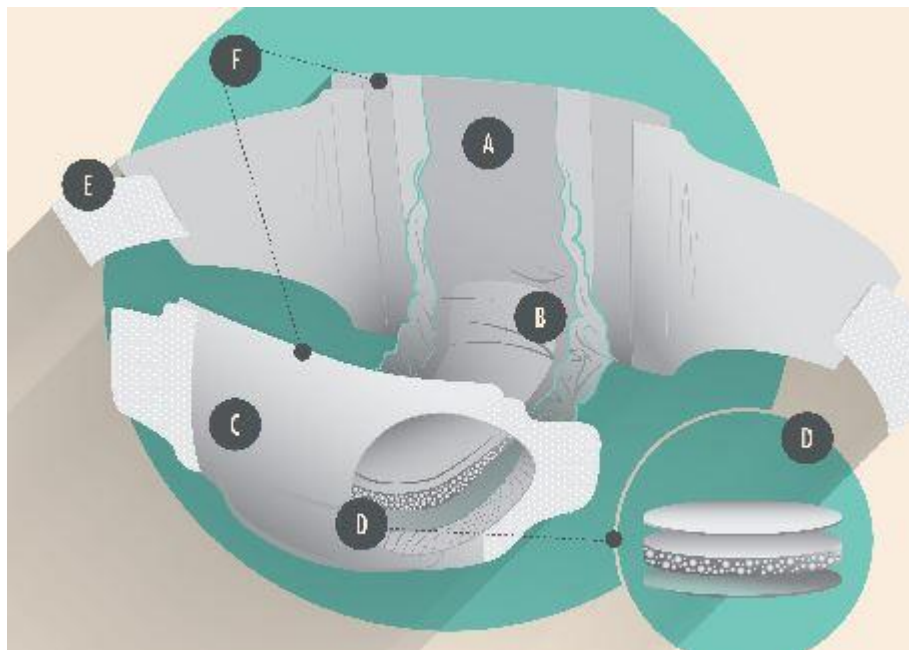
Figure 39 Schematic of the layers of construction of a disposable nappy. Source EDANA Baby diapers and nappies from raw materials to your home.
