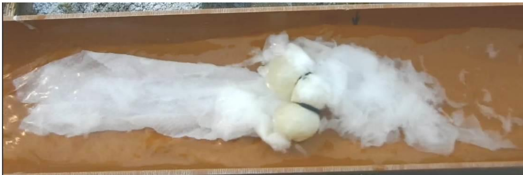
Photograph D 5 Accumulation of material on snagged sample (representing a fail)
