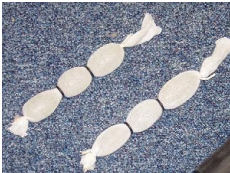
Photograph D 2 Examples of the simulated faecal solid
