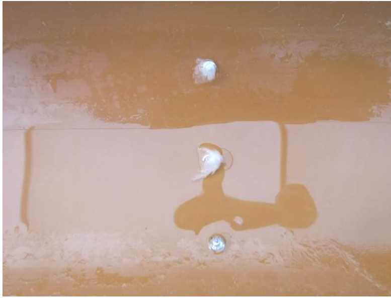
Photograph D 4 Small traces of sample remaining (representing a pass).
