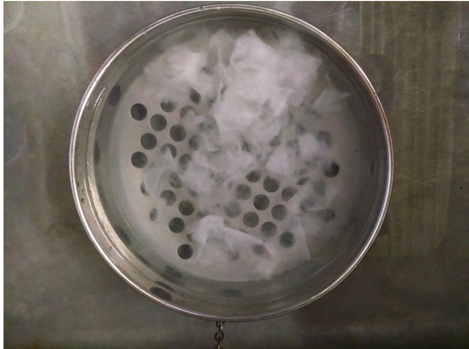
Photograph C4 The contents after being poured into the submerged sieve
