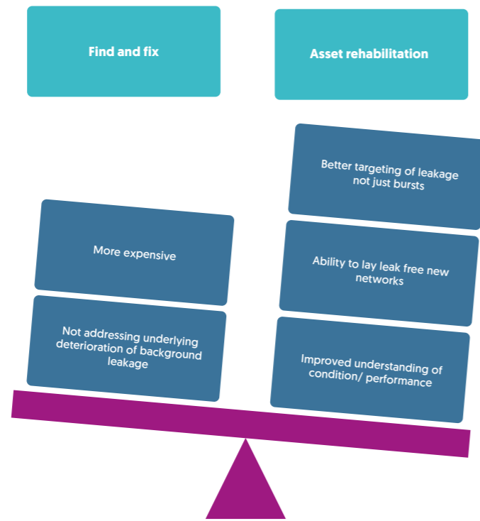
Figure 4.3 – The balance between operational and capital solutions for a future with an asset management focus
